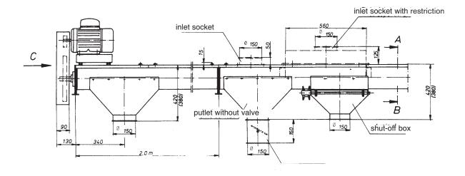
TS 1702: Conveyor capacity up to 17.000 kg TS 2003: Conveyor capacity up to 20.000 kg
