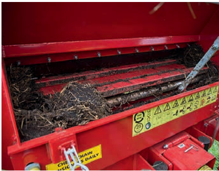
You can access the tensioner for the moving floor under the flap at the front.
