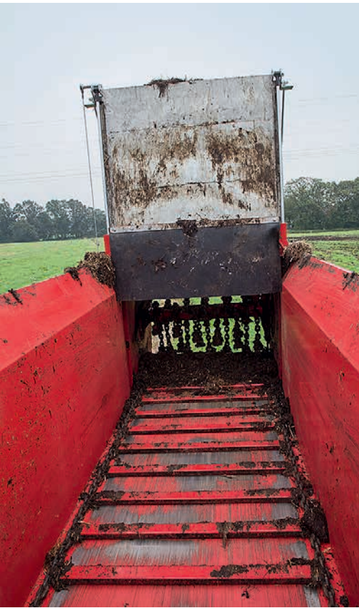
A rubber section on the slurry door ensures no manure is thrown towards the tractor.
