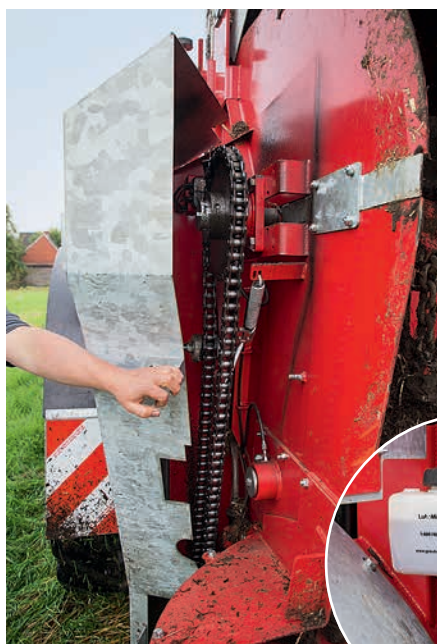
Once two chains are connected to the slurry door, this can be used to lift the spreading hood into its service position. There are 22 chains dispersed across four rows.
