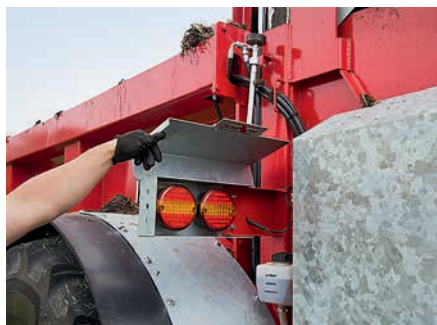
Guards connected to the slurry door protect the road lights.
