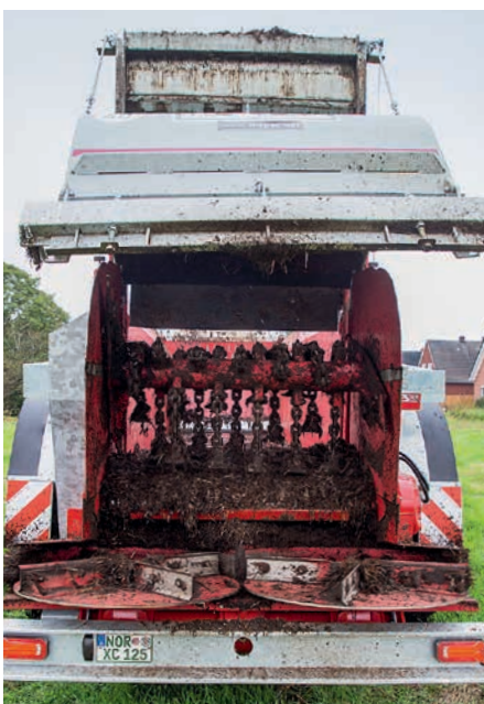
Once two chains are connected to the slurry door, this can be used to lift the spreading hood into its service position. There are 22 chains dispersed across four rows.
