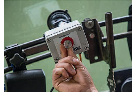
The speed of the spreader floor is controlled using the dial on the in-cab box.
